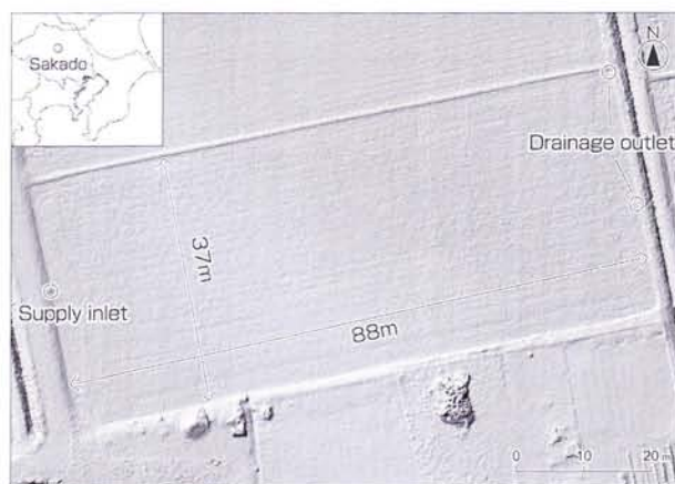
Fig. 3 Location map and test site (Background : shaded-relief map created from DSM (ground resolution 5 cm) before soil puddling).
